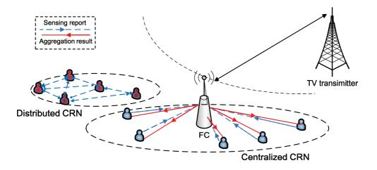
Fig. 1. Distributed CRN and Centralized CRN
